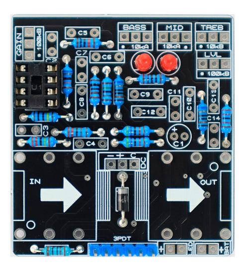
First of all place the IC sockets (without the ICs). Pay attention to the orientation! The small notch in the socket should be oriented as indicated in the PCB.
